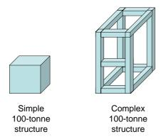
The Marine Energy Challenge used engineering experience and a build-up of unit costs, as well as quotes for the construction of the whole unit from experienced fabricators. Both approaches are needed. The first is simpler and allows the trade-offs between cost and performance to be made more readily and the second is suited better to refined designs.
