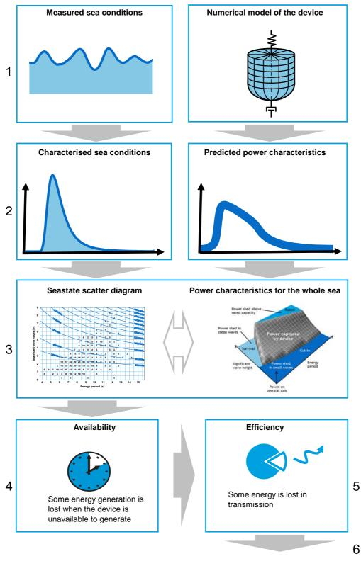
Figure 3.1 Simplified process for calculating the energy production of a marine energy project
